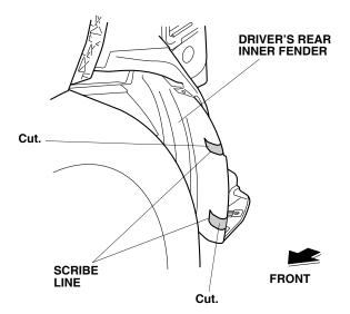
20. Using a utility knife, cut off the tab from the driver's rear inner fender as shown.
