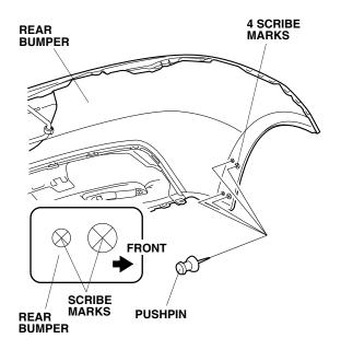
13. Using a pushpin, pierce the center of one scribe mark on the bottom of the rear bumper as shown.
