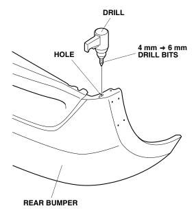
Drill the four holes on the rear bumper with a 4 mm drill bit.
