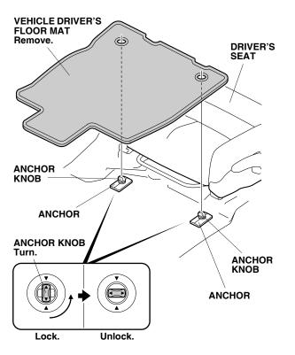
Install the rings in the driver's all-season floor mat over the anchors. Turn the knob on each anchor 90° to secure the driver's all-season floor mat.
