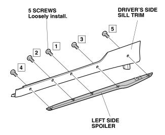
10. Tighten the middle screw 1 loosely installed in step 9.
