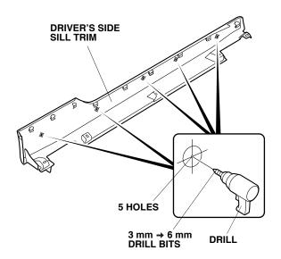
Using isopropyl alcohol on a shop towel, thoroughly clean the side sill trim where the side spoiler will attach.
