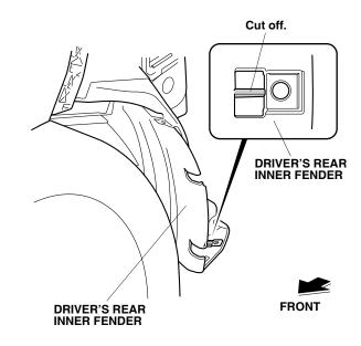
21. Install one spring nut over the hole in the driver's rear inner fender.
