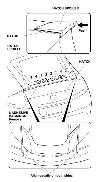
20. Using the palm of your hand, firmly press the hatch spoiler to the hatch for 30 seconds.
