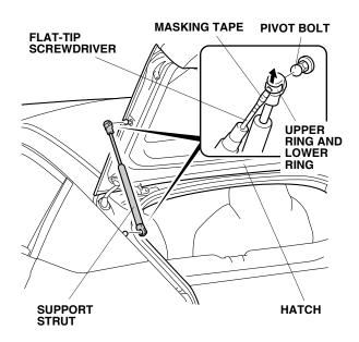
2. With an assistant holding the hatch open, use a flat-tip screwdriver wrapped with masking tape to release one upper ring and one lower ring. Remove the left support strut as shown.
