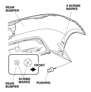
13. Using a pushpin, pierce the center of one scribe mark on the bottom of the rear bumper as shown.
