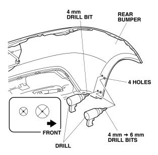
16. Enlarge the two front holes in the rear bumper with a 6 mm drill bit. Remove any burrs.
