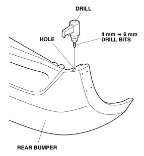
Drill four holes in the rear bumper with a 4 mm drill bit.
