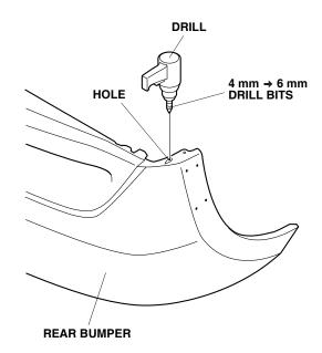
15. Drill four holes in the rear bumper with a 4 mm drill bit.
