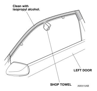
7. Remove the adhesive backings from one sealer A and one sealer B and attach them to the door sash as shown.
